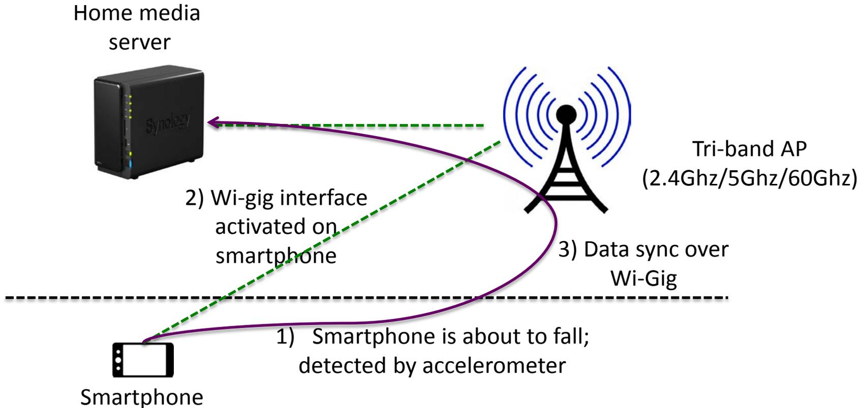
**Step 2:** Accelerometer on the phone detects a fall and it instantly turns on the Wi-Gig interface.
