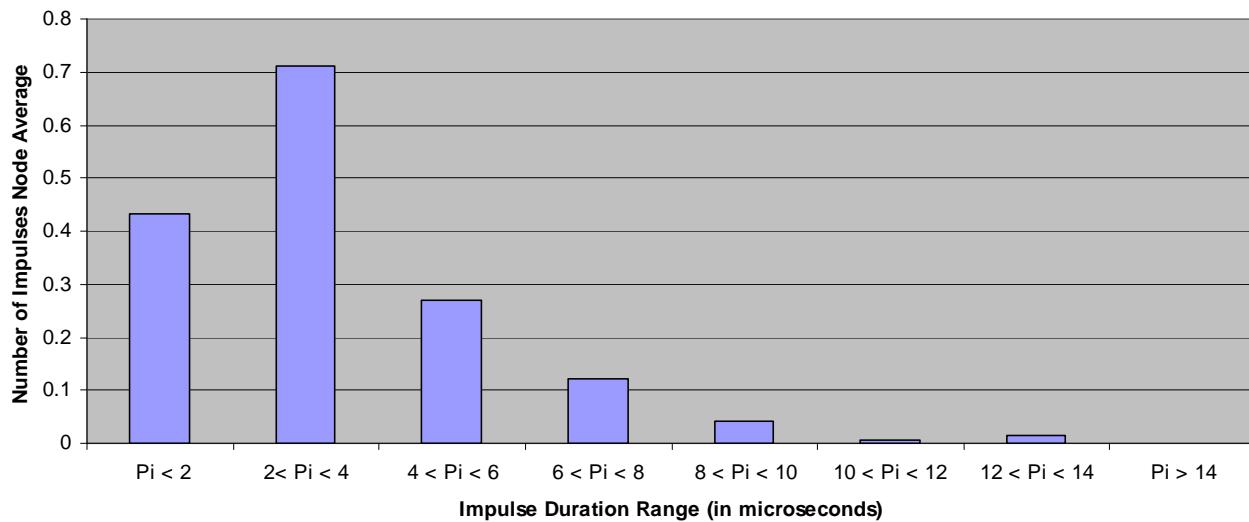
**Figure 4 - Impulse Duration Characteristics**
