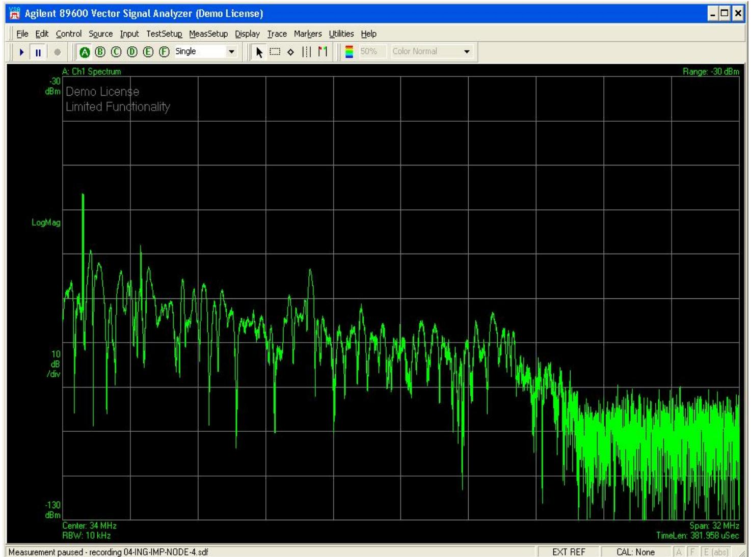
**Figure 1 – Upstream Spectrum Capture Showing Impulse**
