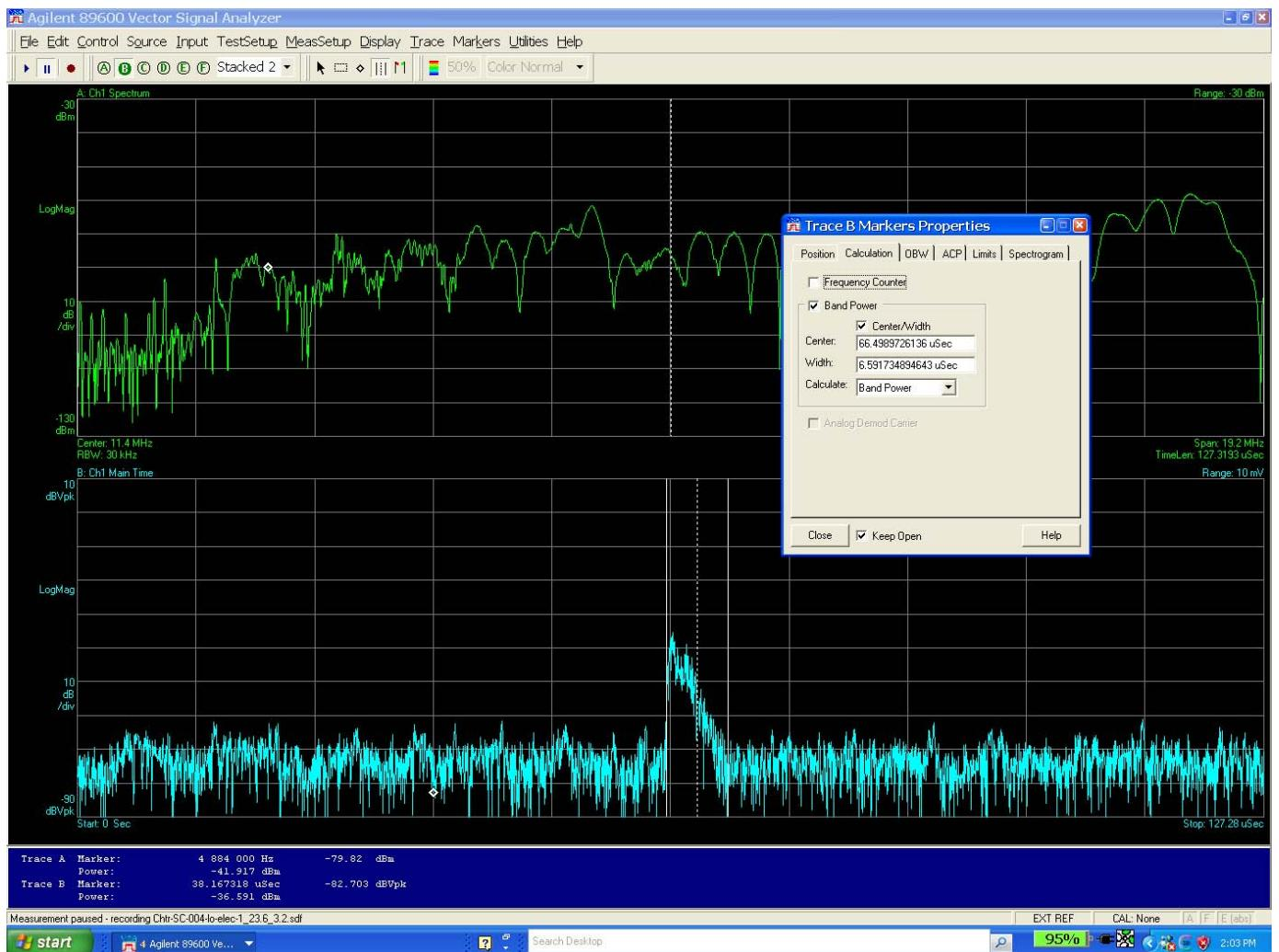
**Figure 3 - Typical Impulse in time and frequency**
