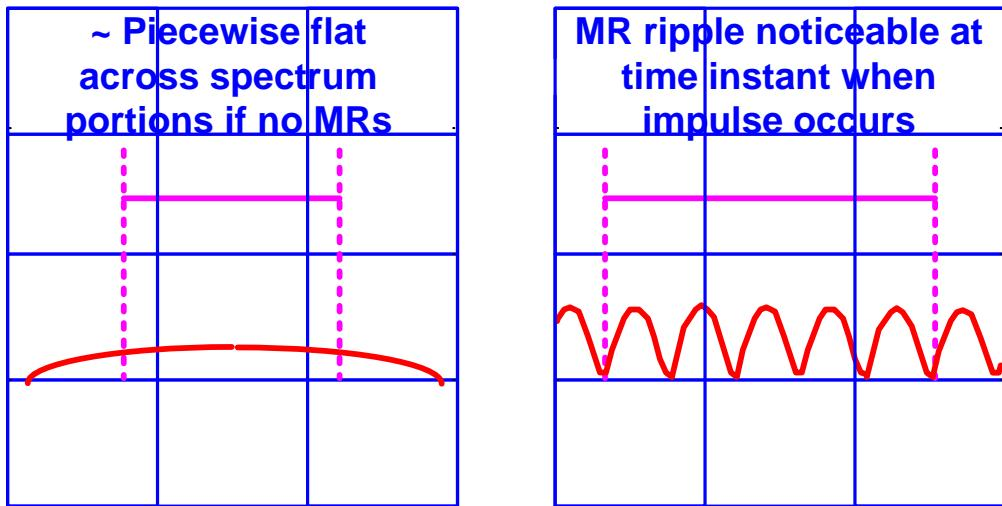
Figure 6 Frequency view of impulse noise affected by micro-reflection
